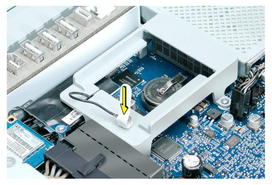
7. With a plastic tool, thumb, or finger, push the battery in the direction of the arrow to free the battery from the metal clip.
